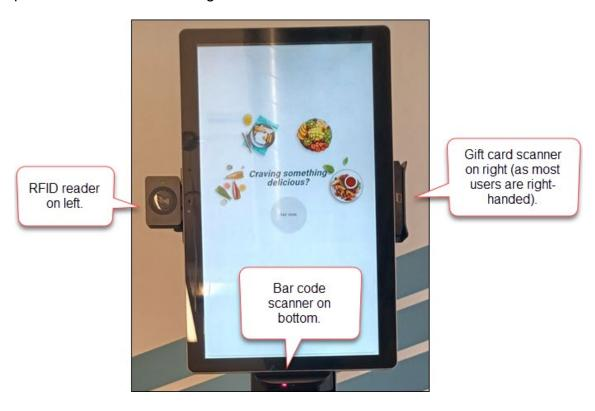
To properly orientate the touchscreen monitor when connecting the accessories, note that the word "Elo" is on the right side when viewing the monitor from behind.
