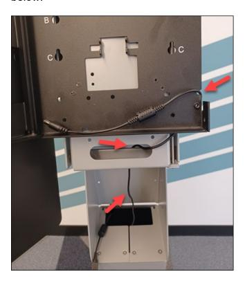
Connect the power cable to the touchscreen monitor power port.
