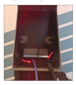
Secure the printer mount to the stand via the two mounting holes at the rear of the stand.
